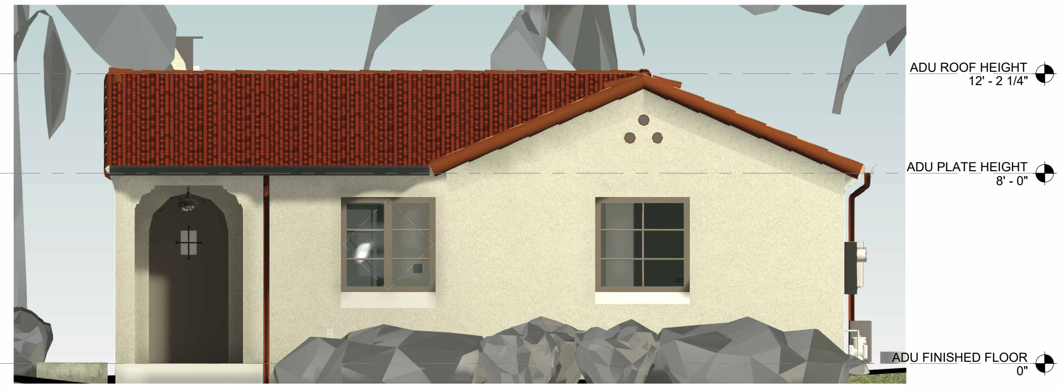
SOUTH ELEVATION W/O CHIMNEY SCALE: 1/4" = 1'-0"
